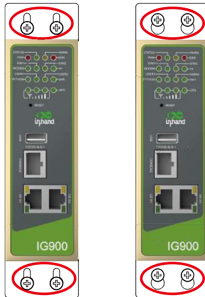
Figure 3-4 Wall mounted installation diagram
