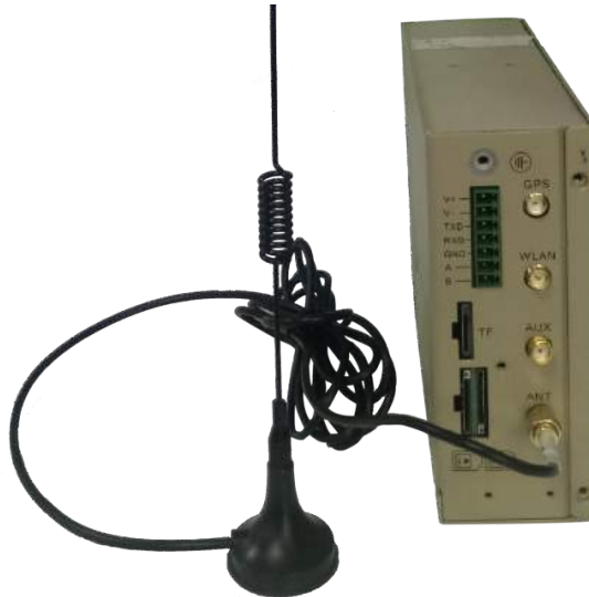
Figure 3-6 Installing an Antenna
