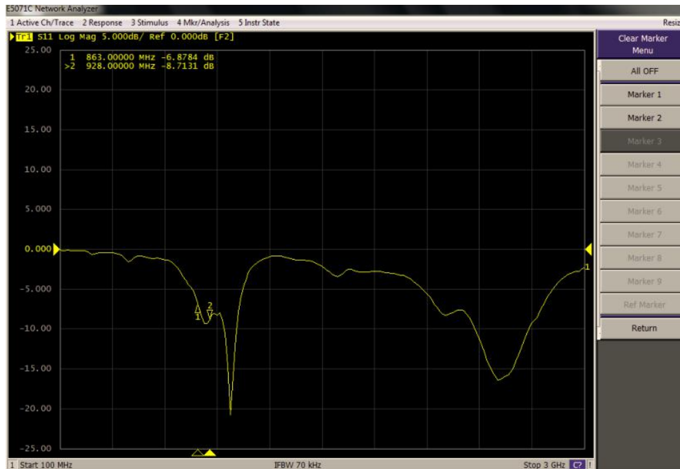
Figure 9 | LoRa Antenna performance
