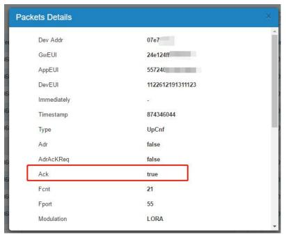
Ack is "true" means that the device has received this packet.
