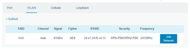
2. Select one access point and click "Join Network", then type the password of the access point.
